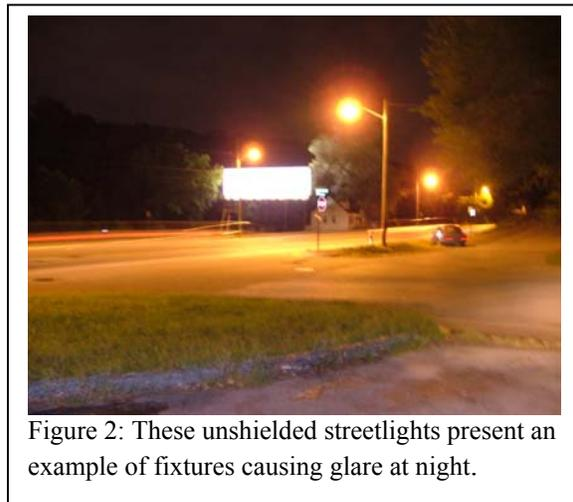
Figure 2: These unshielded streetlights present an example of fixtures causing glare at night.
