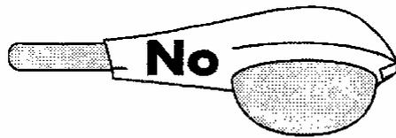
Same fixture as above mounted incorrectly – defeating the horizontal mounting design. The fixture now produces direct glare, and can also produce uplight at steeper mounting angles.
