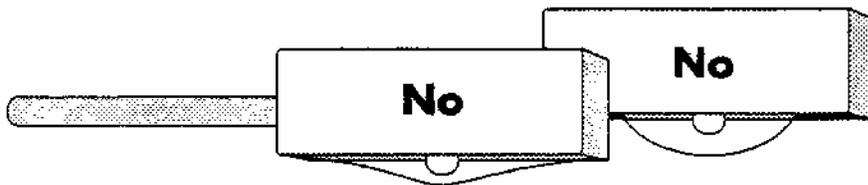
Known as just "Cutoff" Center "drop" or "sag" lens with or without exposed bulb, produces direct glare.
